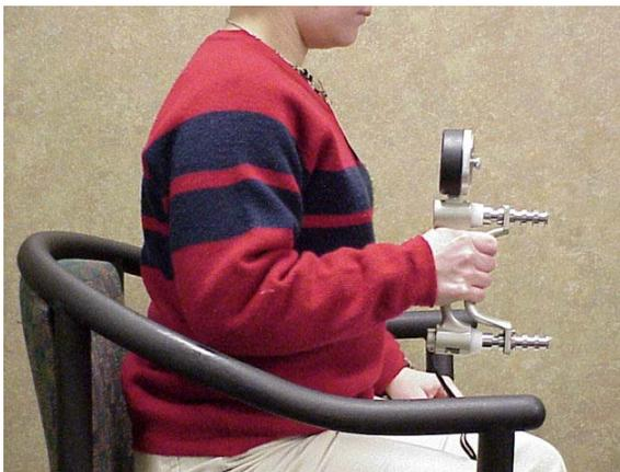
Figure 1. - Jamar® Hydraulic Hand Dynamometer Positioning
